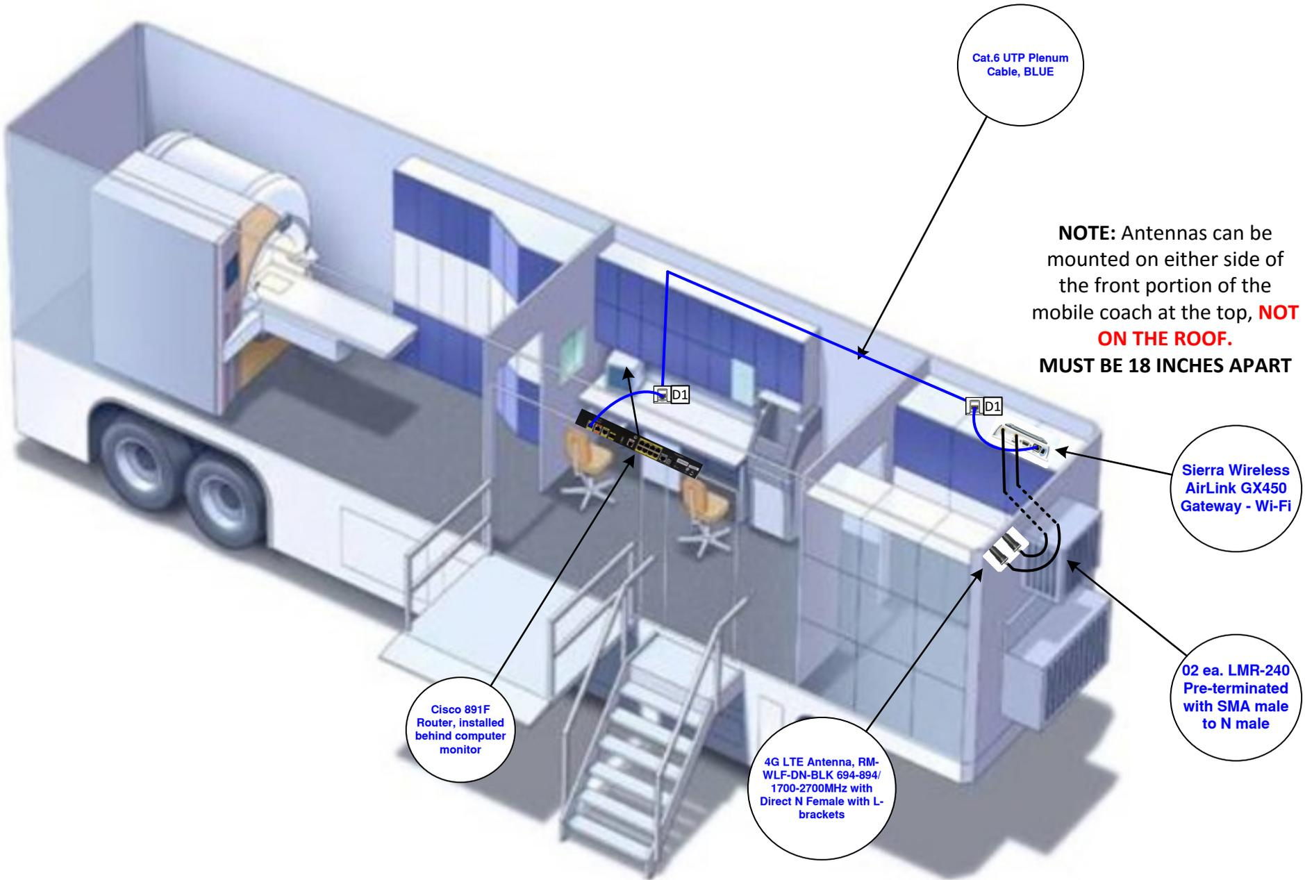
**NOTE:** Antennas can be mounted on either side of the front portion of the mobile coach at the top, **NOT ON THE ROOF.** **MUST BE 18 INCHES APART**
